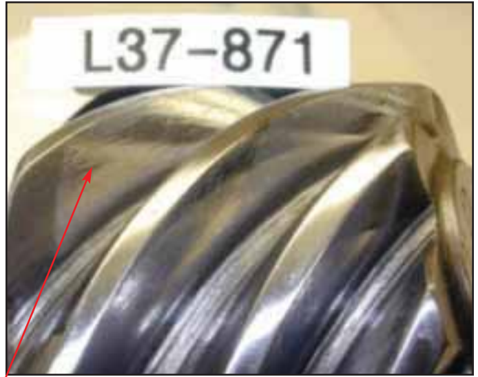
Pinion gear - original machine marks still present.
