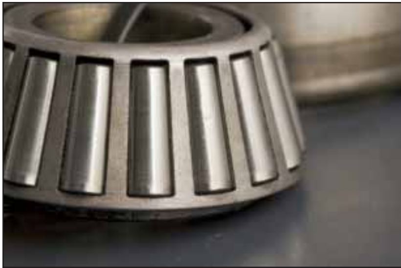
Pinion tapered roller bearing in like-new condition.
